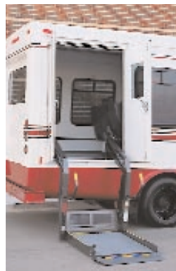
Optional paratransit lift equipment available either in front or rear of axle
